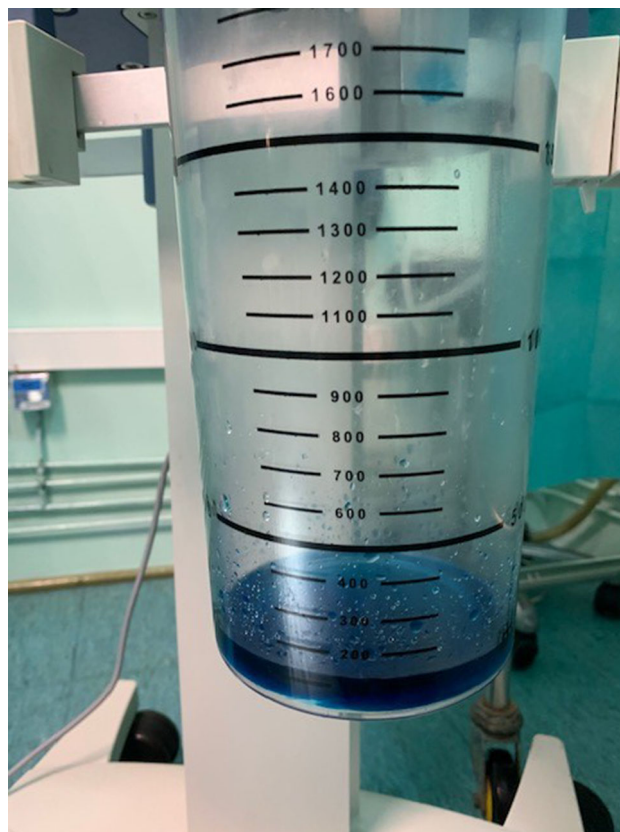
Fig. 7 Photograph of the aspirator's collector after injection of substrate during constant motion of the cannula. The collector is clearly filled with part of the colored injected substrate
